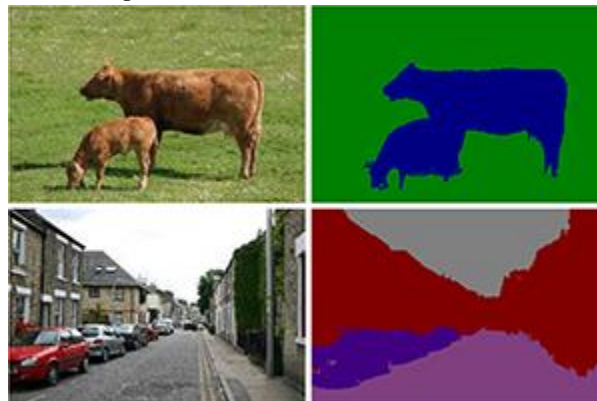
Figure 2 Input And Output of A Semantic Segmentation Algorithm
